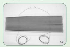
1.7 Inspect the cord bushings in the fabric and if broken or worn, replace with supplied bushings. Carefully thread cord through bushing noting that the cord coming from the left will run down through the left side of the material. The cord coming from the right will run down through the right side of the fabric.
