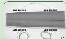
3.7 Inspect the cord bushings in the fabric and if broken or worn, replace with supplied bushings. Carefully thread cord through bushing noting that the cord coming from the left will run down through the left side of the material. The cord coming from the right will run down through the right side of the fabric.
